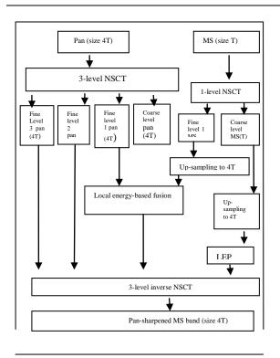
Fig.7.Proposed Method based on NSCT using LEP (local edge preserving filter).
