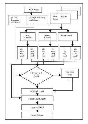
Fig.4. Flow chart of the Existing Method to get Pan sharpened Image using NSCT.
